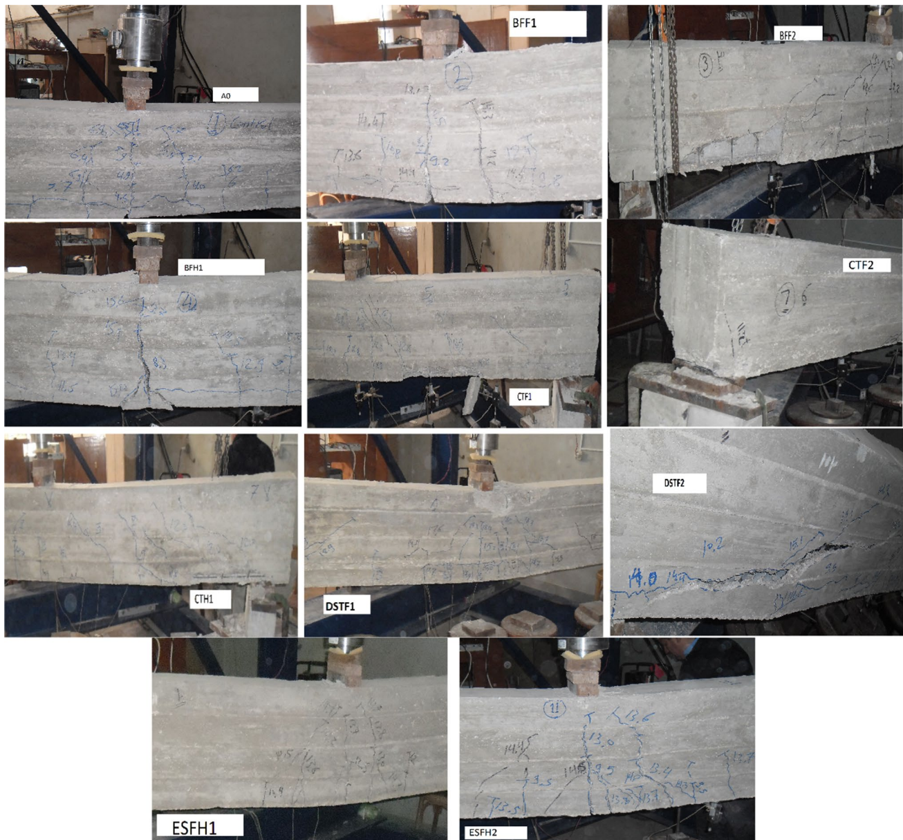
Fig. 7 Modes of failure for specimens
